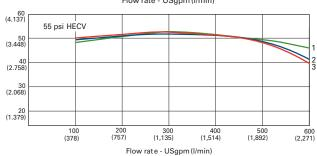
Curve 1 Control pressure with 100 psi (6.895 bar) inlet pressure
